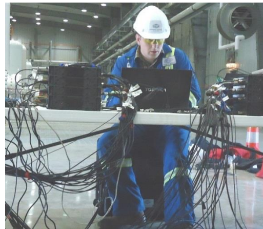
Figure 1. Example of data collection equipment required to measure transients' vibrations on hundreds of simultaneous test points
