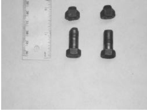
Figure 1. Broken coupling bolts
