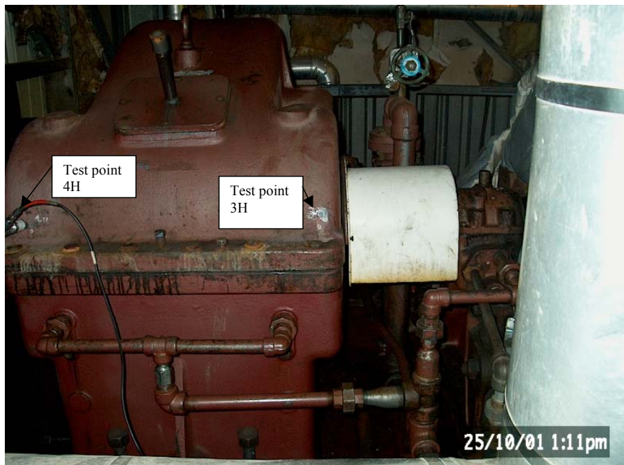
Picture 1: High speed side of the box, Test Points 3 and 4: (Turbine to the right)
