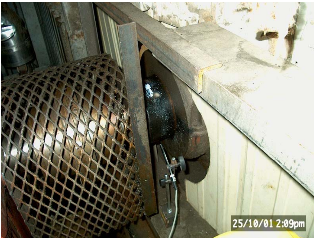
Picture 3: Optical pickup on the low speed shaft. Once per turn mark was put on the shaft while it was running.
