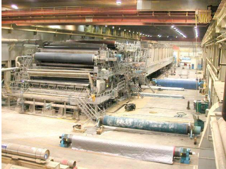
Figure 1. The paper machine viewed from the former section towards the dryer end, showing the front or tending side of the machine. To the right of the paper machine can be seen the roll and felt laydown areas needed for the shutdown. Monitoring equipment was located just beyond the blue roll at the wet end of the dryer, and at the far end of the dryer.
