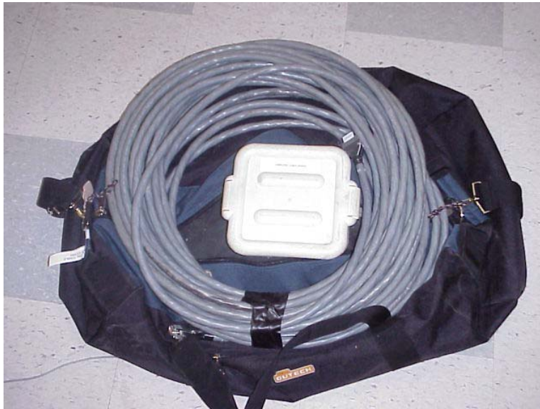
Figure 4. The 12 channel umbilical cable – 30 metres in length with serial connector ends.
