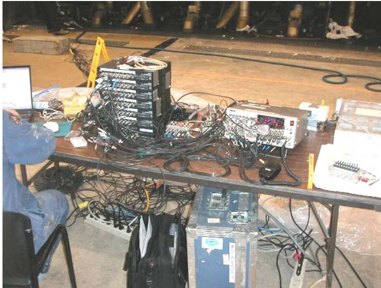
Figure 2. Former and press data acquisition equipment monitoring 56 vibration and 4 tachometer channels.
