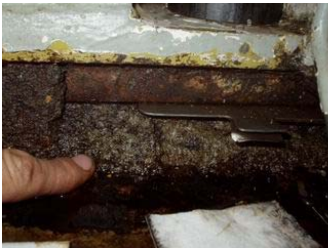
Figure 6: Photo of actual grout connection. Finger points to location where most relative motion can be felt or seen.
