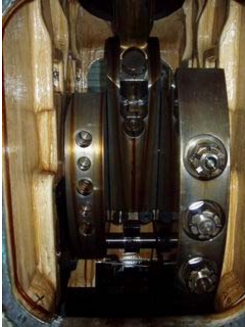
Figure 7: View of engine crankshaft throw #4 with web deflection gauge installed
