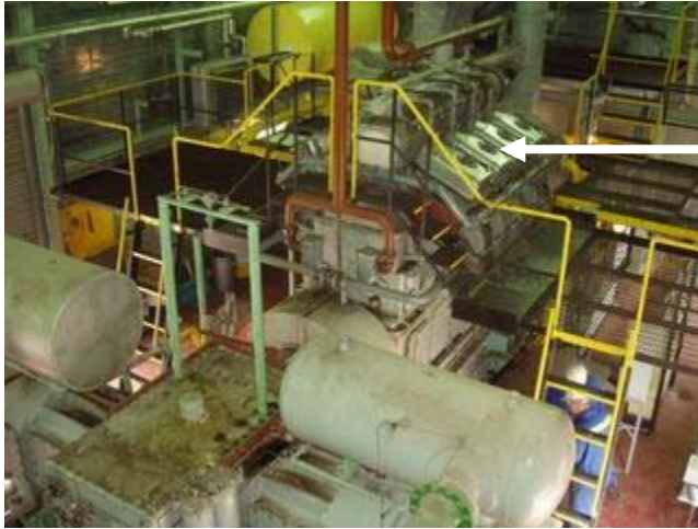
Figure 1: Picture of Engine-Compressor, compressor in foreground. Note the beautifully polished valve covers on the engine.
